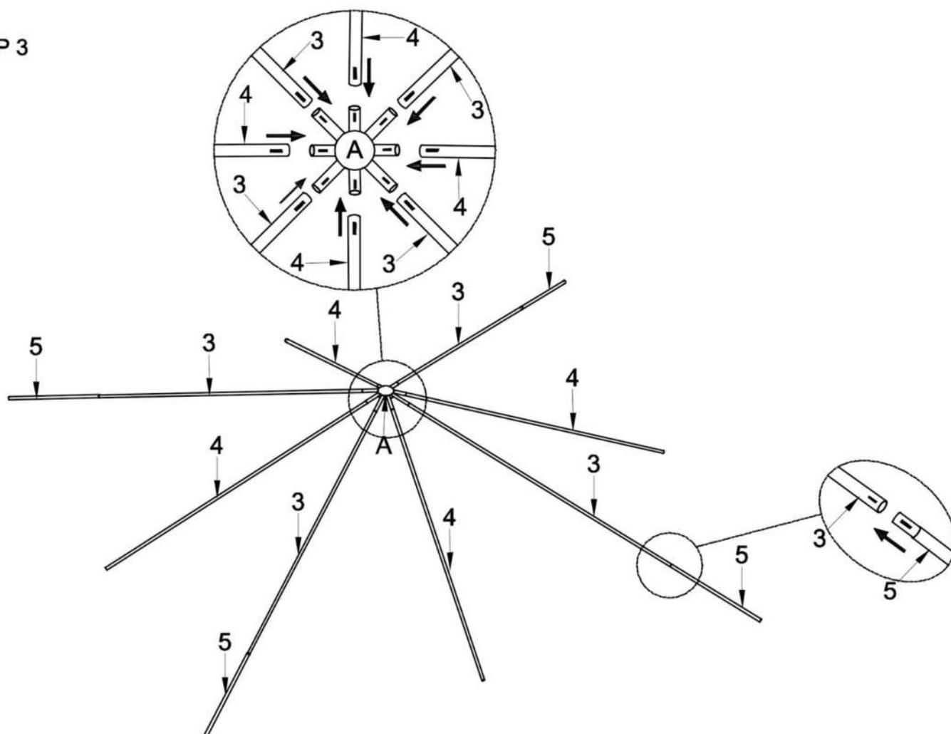
4. To attach the roof to the frame, insert all the poles through the corners and middle of the metal bar (2). Secure each pole with a screw (X3) and bolt.
